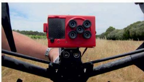
Fig. 2. A close up of a five band multispectral camera mounted to an unmanned aerial vehicle (UAV).
